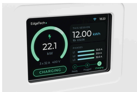
The display: power, session energy, current per phase, state
