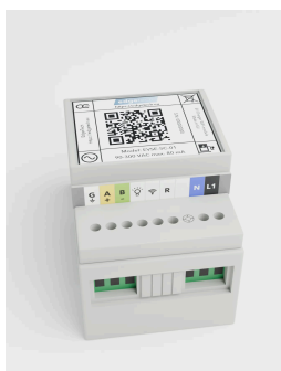
Terminal side: RS485 bus, supply
