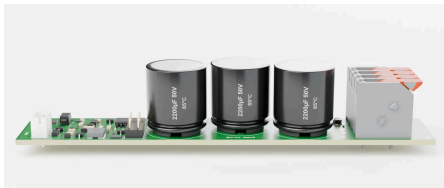
Tallest parts 20 mm above the board
