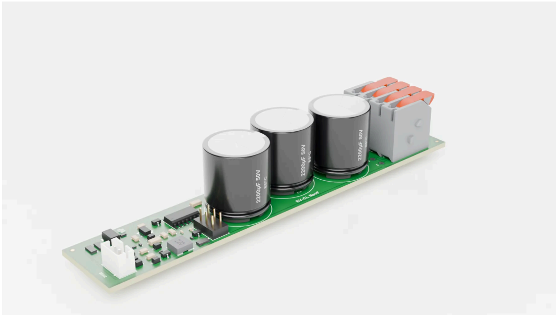
122 × 22.5 mm board: controller connector on the left, reserve capacitors in the middle, lock terminal on the right
