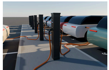
Concept render, design C: two sockets per pole, one toward each row
